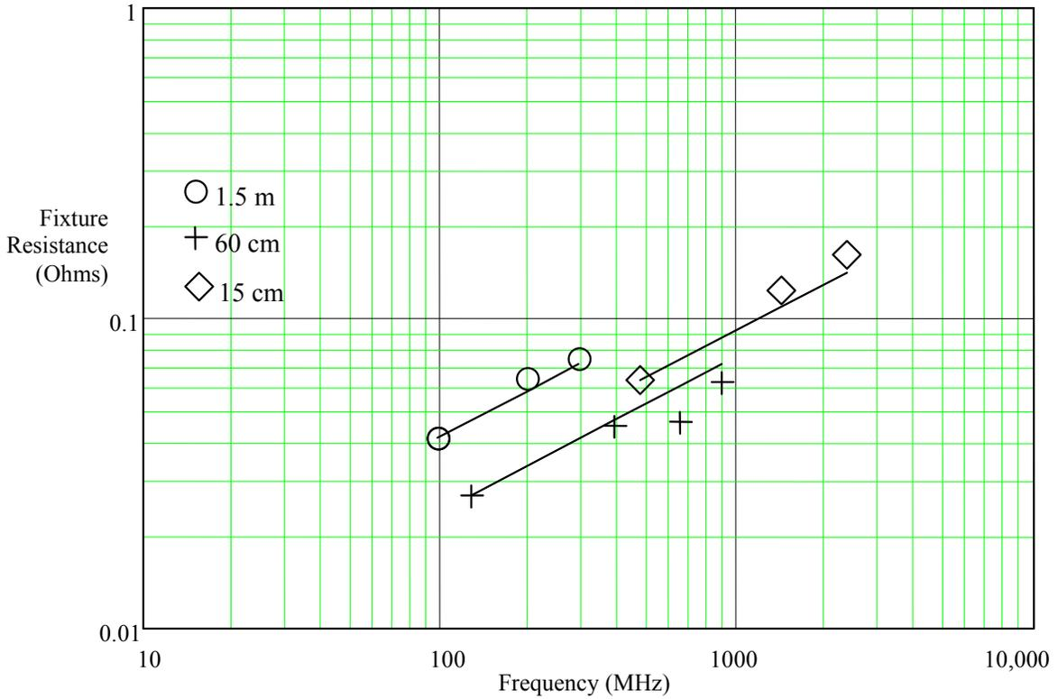
Fig. 4. Calculated fixture resistance for three resonant lines with skin depth rule applied to each result.
