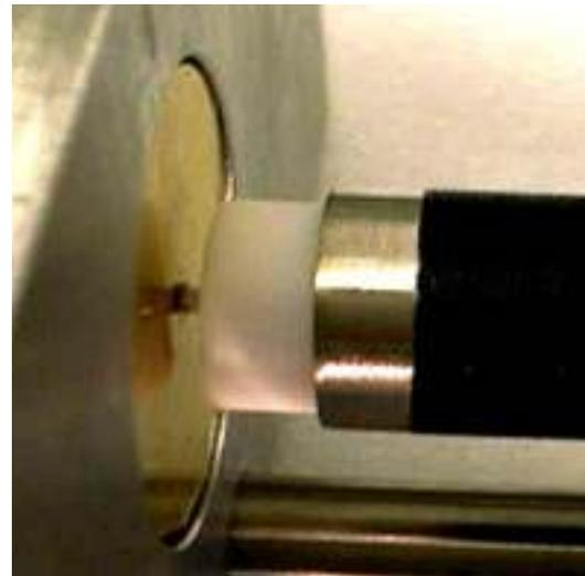
Fig. 10. EIA size 0504 device captured between center conductor and shim of 15 cm line. Note rhodium plating on outer conductor and solid Teflon bushing.
