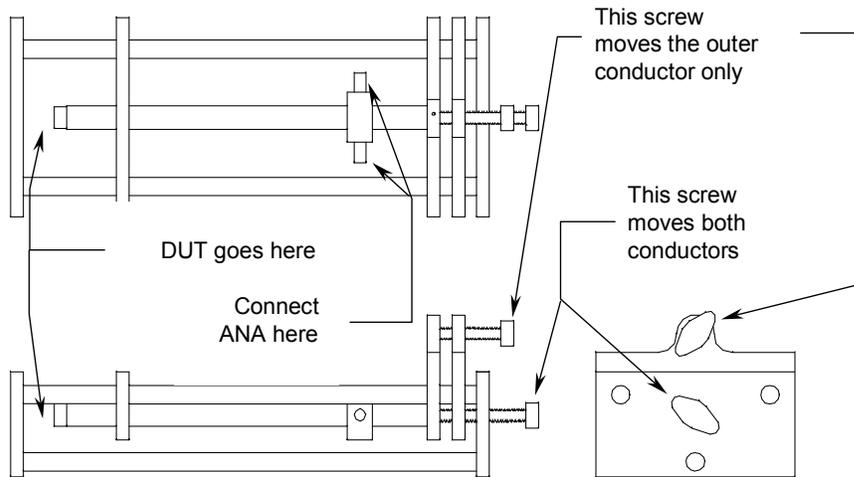
Fig. 9. Plan view of 15 cm resonant line. The DUT is placed onto the center conductor and the lead-screw that moves both conductors is turned until the DUT is clamped between the center conductor and shim. The outer conductor is then brought into contact with the shim by turning the lead-screw that moves the outer conductor only.
