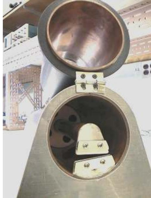
Fig. 6. Wedge fixture of 1.5m SC line. Note circular waveguide section, hinged to the support, at top.
