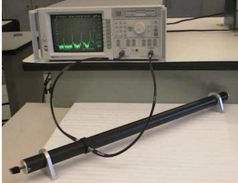
Fig. 7. 60 cm OC resonant line, connected to HP 8714C RF VNA. The lead-screw, left foreground actuates a dielectric rod, which drives the center conductor. The DUT is inserted through a port in the opposite end. Note the resonances displayed on the VNA
