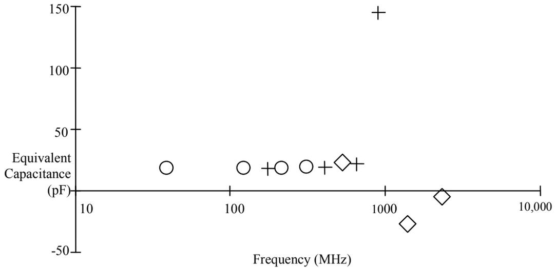
Fig. 11. Equivalent capacitance of 18 pF MLC, measured on three different lines.
