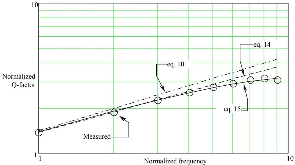
Fig. 2. Normalized Q-factor vs. normalized frequency of Boonton 34A resonant line, S/N 176. Circles represent measured data points. Lines represent interpolation equations, forced through  $Q(f_0)$ .
