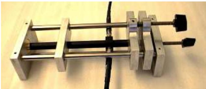
Fig. 8. 15 cm OC resonant line. SMA terminated cables, in foreground and background, connect the line to the VNA. The device is inserted at the left. The top lead-screw, at right, moves the outer conductor, while the bottom lead-screw moves both conductors.
