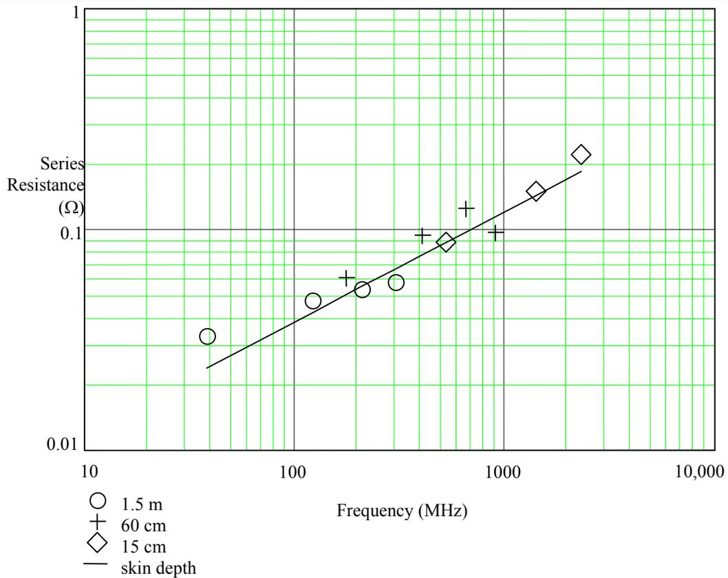
Fig. 12. Series resistance of 18 pF MLC, measured on three different lines.
