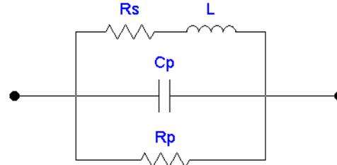
Fig. 13. SPICE equivalent circuit for four EIA size 0805 wire-wound inductors.  $R_s$  ( $1 \text{ }\Omega$ ),  $C_p$  ( $135 \text{ fF}$ ), and  $R_p$  ( $50 \text{ k}\Omega$ ), are the same for all inductors tested, based upon best fit to all measured data.
