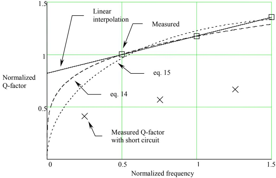
Fig. 3. Normalized Q-factor vs. normalized frequency of Ingalls Engineering 15 cm resonant line, S/N 15c-002. Squares represent measured Q factor of empty line. Solid line is a linear interpolation of measured data, while the dotted and dashed lines are power series interpolations (eqs. 14 and 15). Crosses represent Q-factor of line with a short circuit as a DUT.
