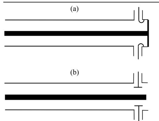
Fig. 1. Loosely coupled transmission lines. (a) Short-circuited termination with inductive coupling. (b) Open circuited termination with capacitive coupling.
