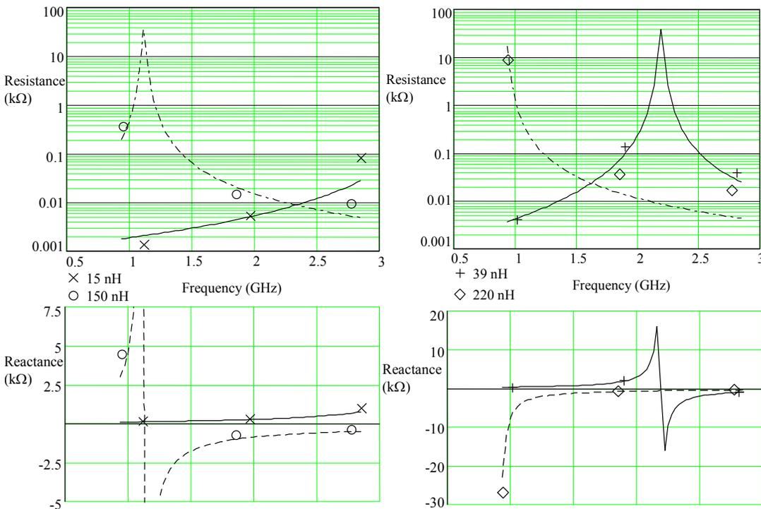
Fig. 14. Resistance and reactance of 15, 150, 39, and 220 nH, wire-wound inductors. Curves are based on measured inductance values and best fit to SPICE parameters for all DUTs, fig. 13.
